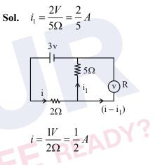
$\therefore$  Current through voltmeter =  $i - i_1$
