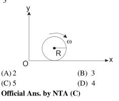
**Sol.**  $L_0$  = angular momentum of shell about O. As shell is rolling so  $V_{cm} = \omega R$  $L_0 = mV_{cm}R + I\omega$  $= 1 \times \omega R \times R + \frac{2}{3}R^2\omega$  $=\frac{5}{2}R^2\omega$
