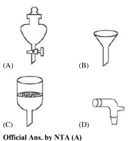
It is used to separate liquid-liquid mixture which is
