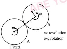
$$\begin{split} \vec{L} &= m\vec{r} \times \vec{v}_c + I_c \omega_0 \\ &= M2Rv + \frac{1}{2}MR^2 \omega_0 \\ &= 4MR^2 \omega + \frac{1}{2}MR^2 \left(2\omega\right) = 5MR^2 \omega \end{split}$$
